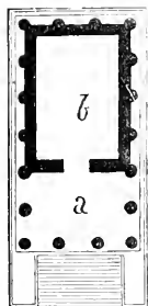
Fig. 535. Ground-plan of a pseudo-peripteral temple.
